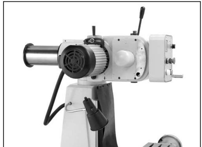
Figure 65. Headstock tilted to 90 degrees.
